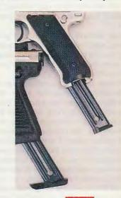
(left) and Mark II (right) magazines are not interchangeable, as the new 22/45 magazine body's angle with relation to the floorplate had to be changed to accomodate the change in grip angle, while maintaining the same feed angle with regard to the receiver body.
